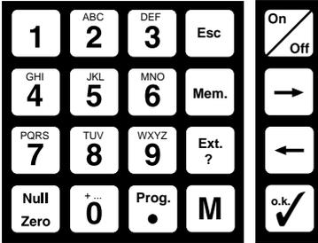
The photometer *NANOCOLOR*<sup>®</sup> 400 D has a 20-part keyboard: 10 numbers and 10 keys with special functions. The whole field is covered with plastic foil and therefore protected against liquid spills and moisture (for example, when a cuvette is spilt). Input verification for all keys increases safety of operation.
